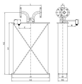
The sensor is manufactured with two internal measurement tubes arranged side by side. In serial or single path sensors, the tubes are connected end to end creating a single path through which all fluid flows. For customization of face to face length and/or special fittings other than the ones listed on this page, please consult factory.
